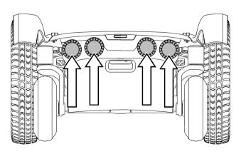
The wheelchair is equipped with reflectors at the front and rear.
