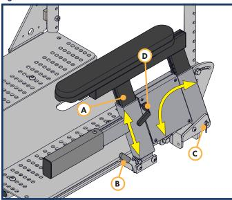
NOTE - To verify that the dual post (fig. 1) and reclining (fig. 3) armrests are properly engaged, pull the end of the armrest up. If it does not move, it is well engaged.
