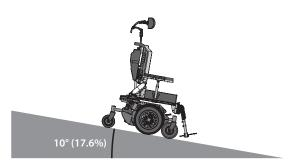
**Figure 1.** Do not use power wheelchair on slope steeper than 10°.
