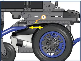
NOTE - For the freewheel position, if levers are difficult to engage or disengage, rock the wheelchair back and forth and/or push against the wheelchair while moving the lever.
